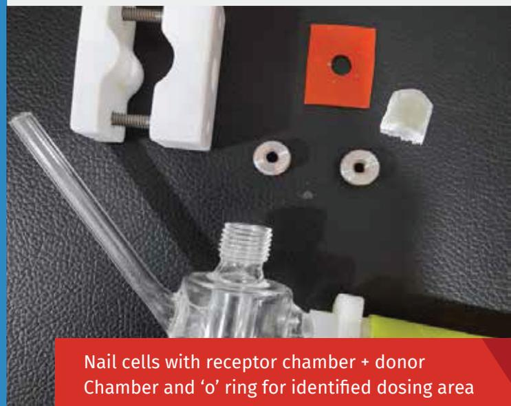
Nail cells with receptor chamber + donor Chamber and 'o' ring for identified dosing area
