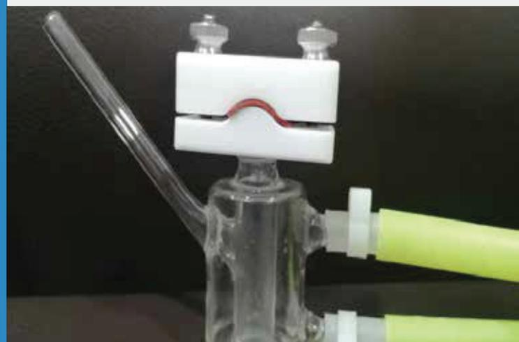
Nail mounted on cell with receptor chamber + donor chamber with water supply tubing to maintain temperature of receptor media throughout the fdc experiment
